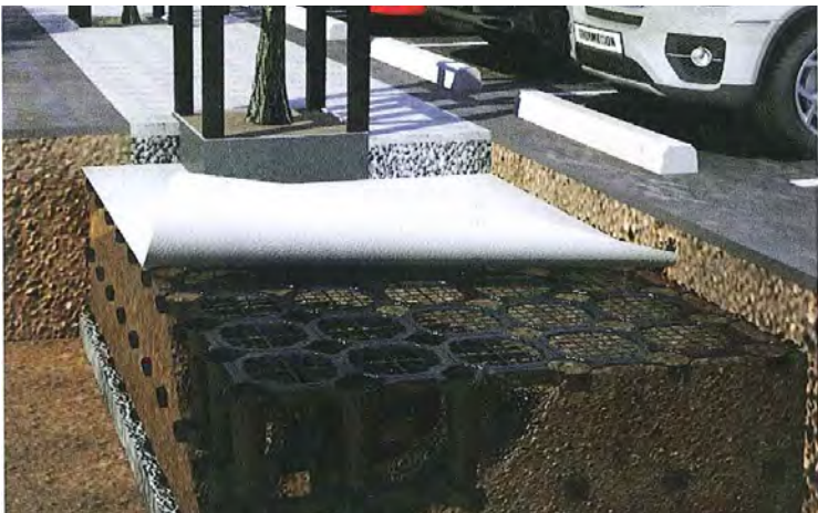
CONTINUOUS SILVA CELL, GREENBLUE OR OTHER MODULAR SYSTEM Image source: GreenBlue Infrastructure Solutions
