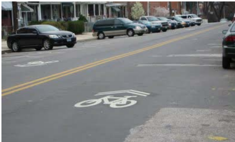
Marked Shared Lanes - Signal to drivers to yield to bicyclists and “share the road” on public streets. These markings also indicate to cyclists the appropriate locations and directions to ride on particular streets.
