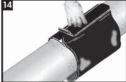
Remove any release liners from the Closure Strip. Centre the closure on the overlapping sleeve. Press down firmly.
