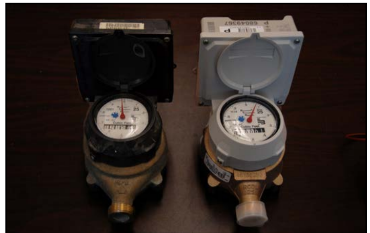
ABOVE: The new meter (at right) looks similar to the current meters (at left) but has a longer battery life.
